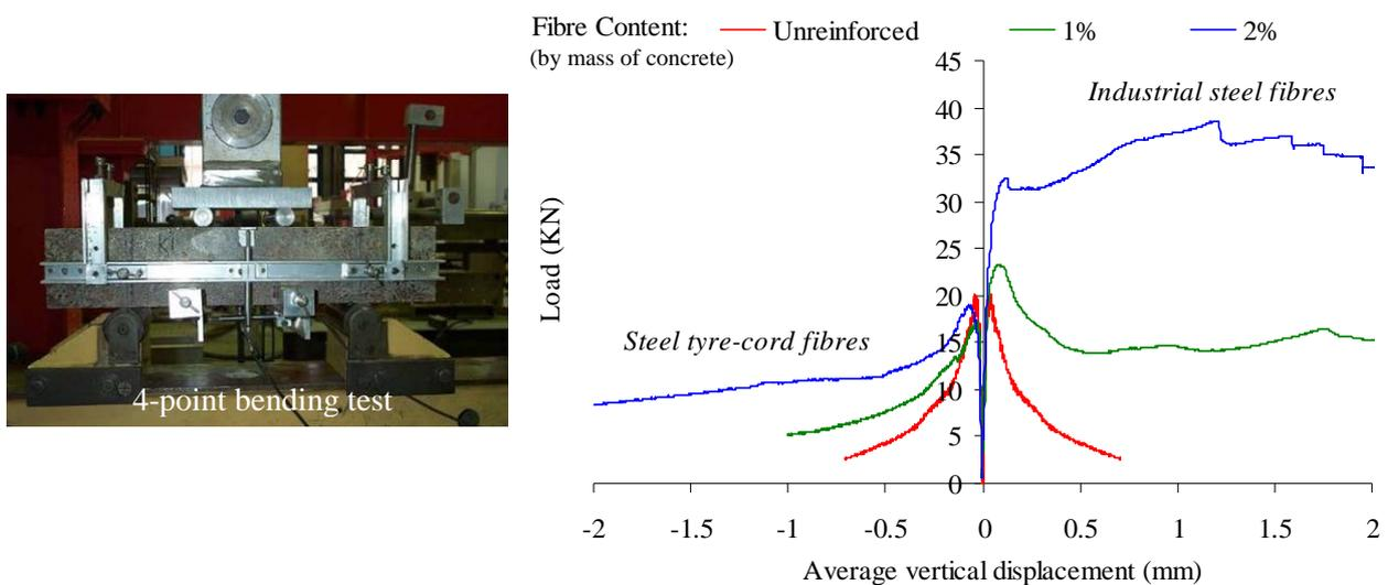
Figure 3 - Bending test results of dry SFRC prisms tested during a pilot study of WP2
