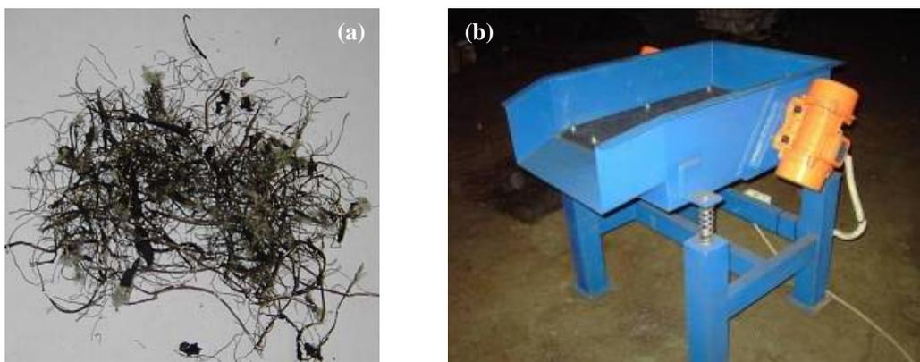
Figure 1 - (a) Unsorted steel tyre-cord fibres recycled from the mechanical treatment of post-consumer tyres, and (b) hardware prototype used for their sorting
