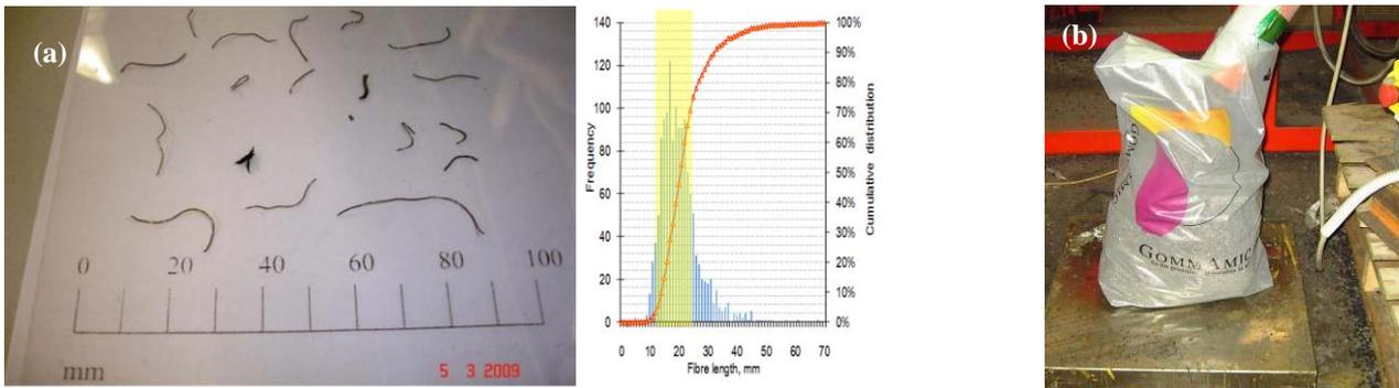
Figure 2 - Steel tyre-cord fibres, recycled from the mechanical treatment of post-consumer tyres: (a) sorted to the project specification, (b) 25kg packaging
