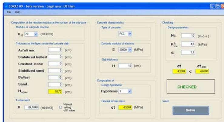
Figure 7 - Design software developed by WP3 for LLRP made with wet and dry SFRC
