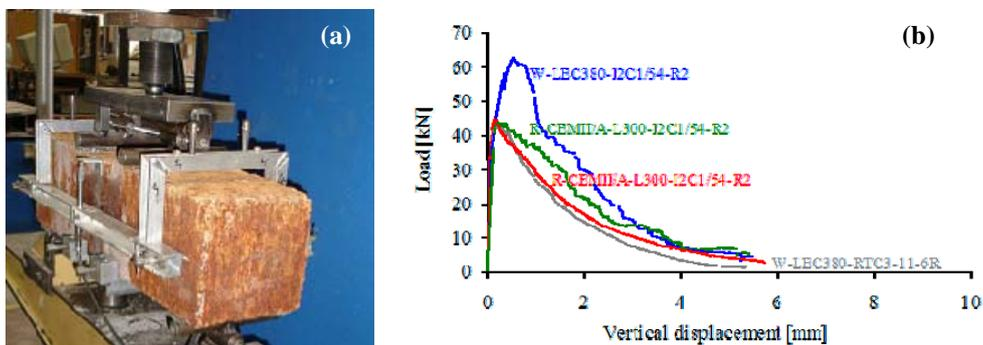
Figure 4 – Bending tests of prisms that initially sustained 5 months of wet-dry corrosion cycles:
