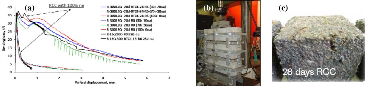
Figure 5 - WP2 experimental work: (a) Flexural behaviour of dry-consistency SFRC mixes made with recycled concrete aggregates, (b) Setup for fatigue bending tests, (c) dry-consistency SFRC samples after 28 days of freeze-thaw testing
